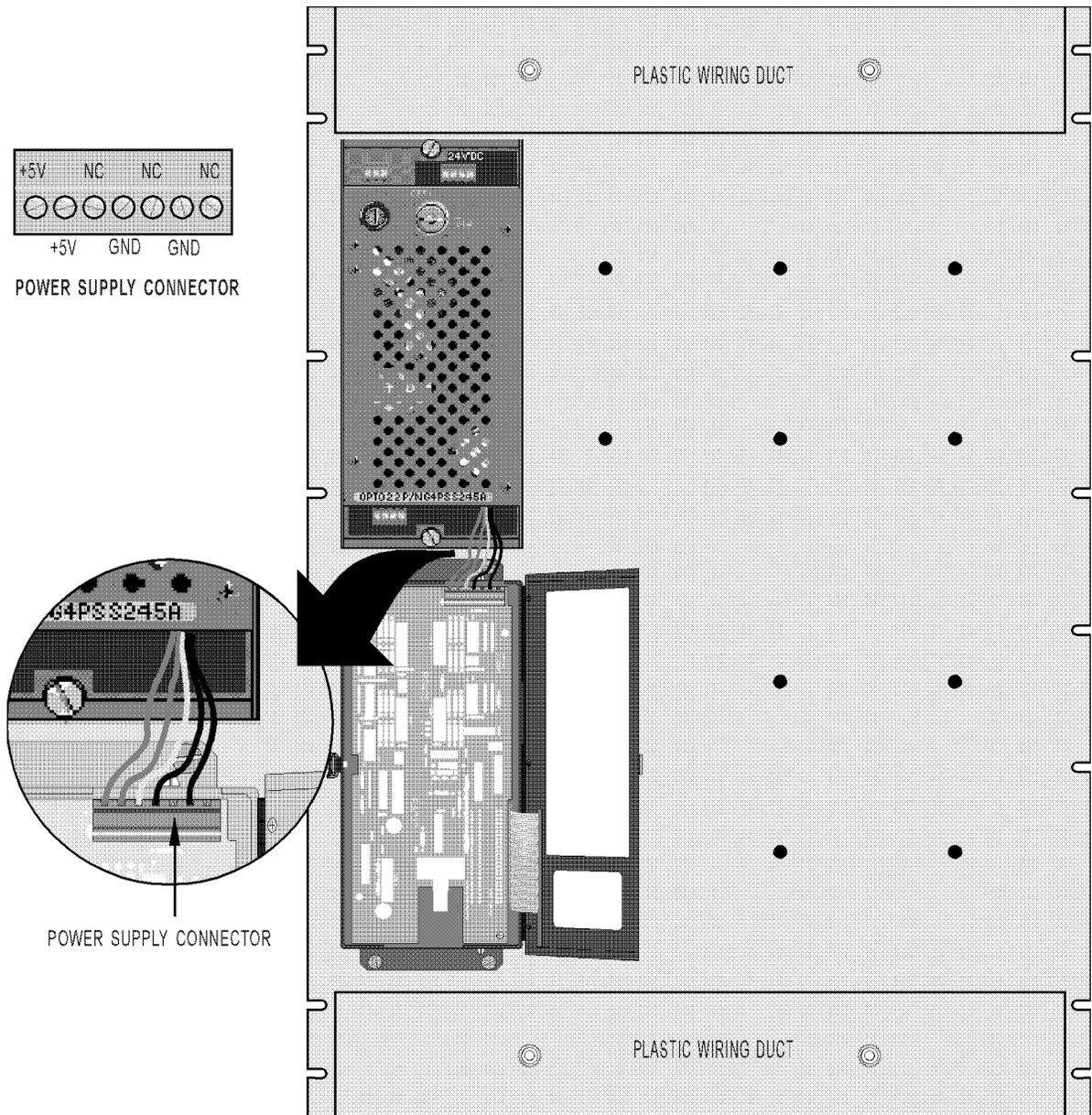
Connecting Power to the G4LC32 Model 200 Processor
