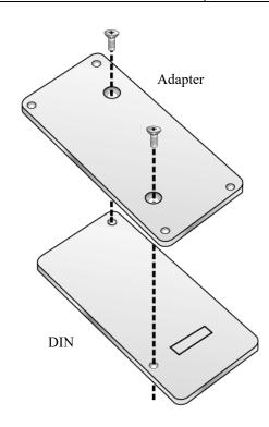
The SNAP-PS5-24DC power supply is shown in this example. Other devices have similar base plates.
