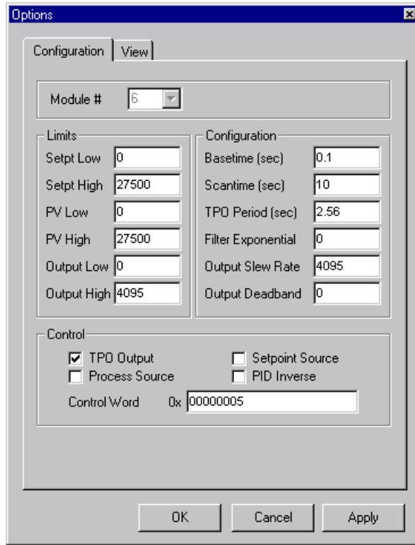
2. In the Limits section, enter setpoint, process variable, and output limit values.
