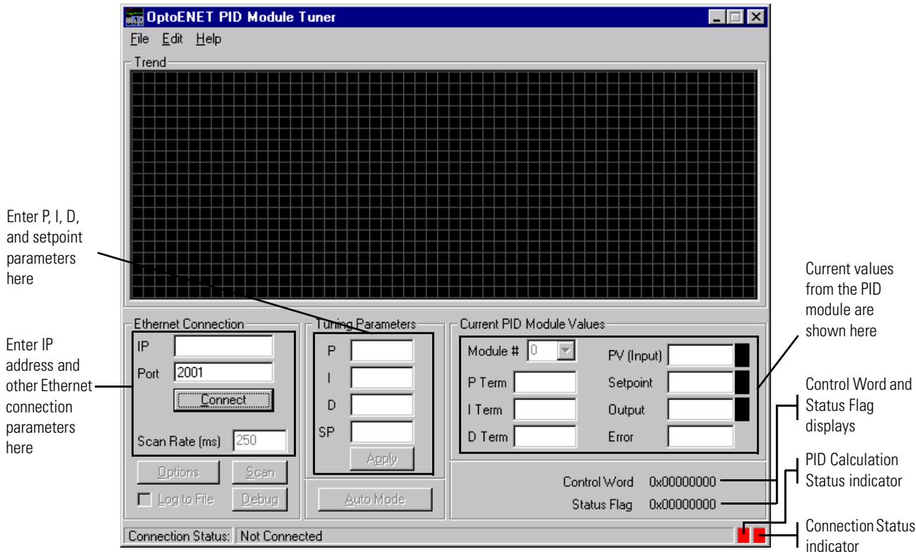
2. In the Ethernet Connection group, enter the SNAP Ethernet brain’s IP address in the IP field.
