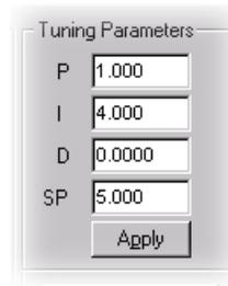
If you need to calculate starting P, I, D, and SP values, use the PID velocity algorithm shown on [page 17](#). You can also start PID calculations using the default P, I, D, and SP values that appear in these fields and then adjust the terms as you tune the PID loop.
