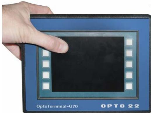
3. While holding your finger on the screen, connect power to the terminal. Release your finger after the Power On Setup screen appears.
