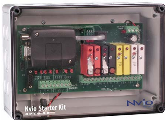
The Nvio Starter Kit unit packages the Sony Ericsson GT48 GSM terminal, Opto 22 G4-series input/output (I/O) modules, and a mounting rack in a compact enclosure.
