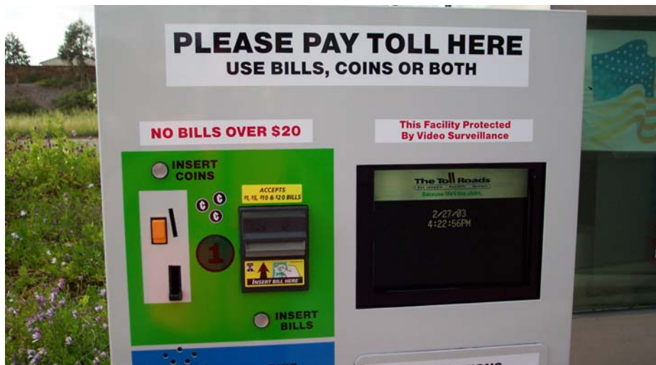
TrafficWerks ATPM allows toll road users to pay with bills, coins, and other means.
