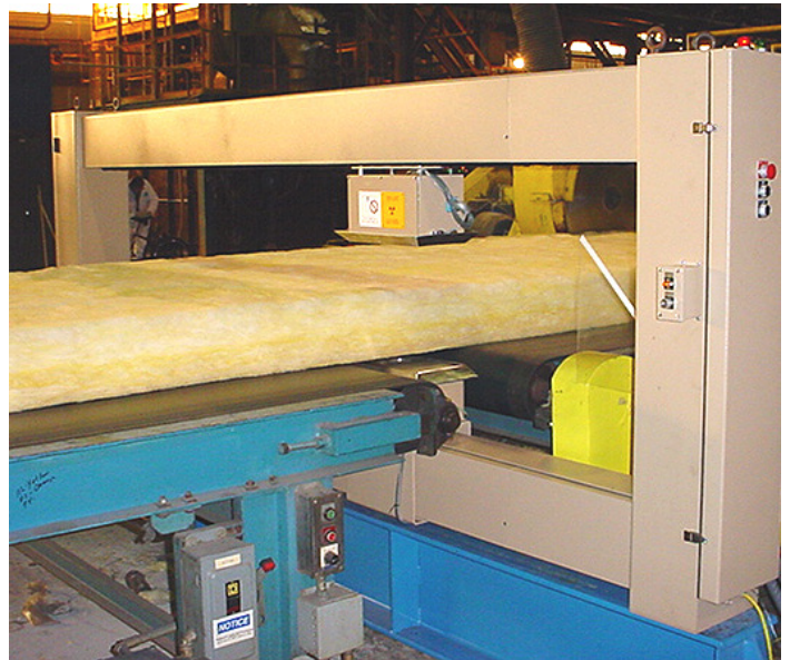
Knauf Insulation's online gauging system measures the density of the product during manufacturing.
