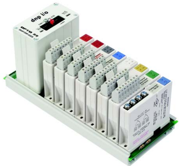
Opto 22 SNAP-DNP-ASDS brain shown with analog and digital SNAP I/O modules on a SNAP mounting rack. Modules and rack are sold separately.
