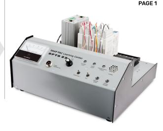
The course uses a learning scenario of a fictional convenience store, with digital input and output devices (lights and door contacts), and analog inputs and outputs (fuel sensors and displays).
