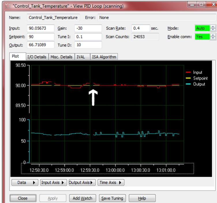
Many PID systems are effectively controlled with Gain and Integral constants only and no Derivative constant. In this example, the Gain and Integral settings are maintaining the temperature at 0.07 from setpoint. To demonstrate the effect of the derivative constant, the resolution of the Input axis was increased to show a 1 percent span. At this resolution, the plot reveals changes of 0.01 degrees F.
