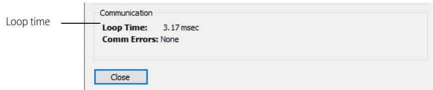
If the loop time was significantly lower when the strategy was stopped, you may be able to improve throughput by minimizing the number of charts that run simultaneously.
