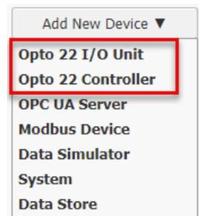
Opto 22 Controller and I/O Unit devices configured in a project. Be sure to add Opto 22 I/O Unit devices at the beginning of your project; making these changes later is much more tedious.
