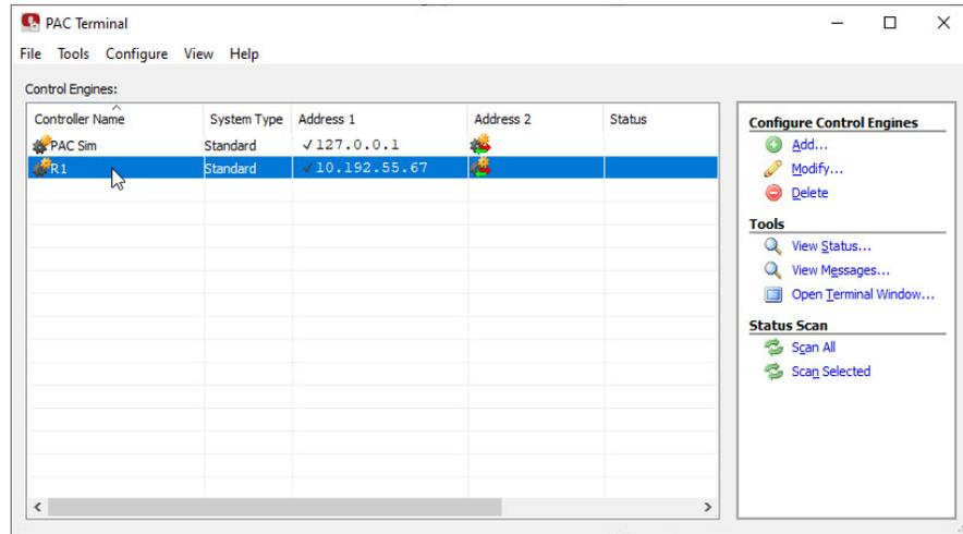
2. While the strategy is running, double-click the controller to inspect the status of the control engine.
