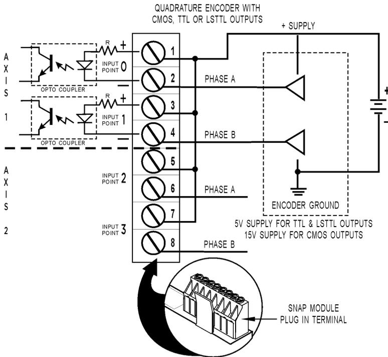
Use the diagram at left for quadrature encoders with **CMOS, TTL, or LSTTL** outputs, and also for encoders with a **pull-up option** (internal pull-up resistors).
