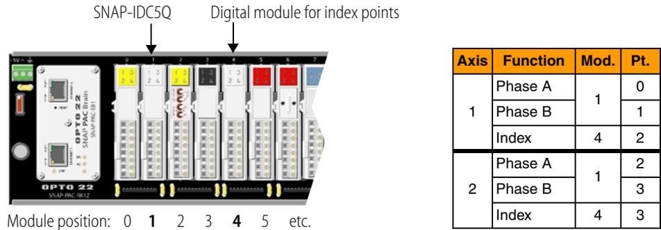
In this example we'll configure the Phase A points, points 0 and 2 (remember, you only need to configure Phase A or Phase B, not both).
