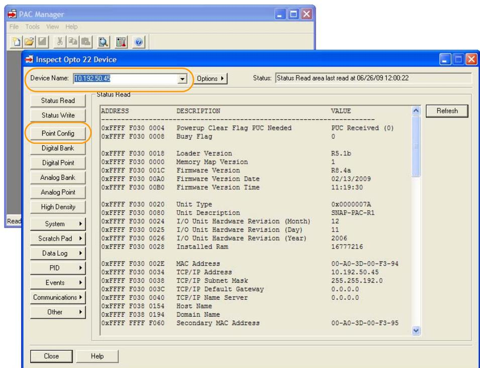
3. In the Device Name field, enter the IP address of the I/O processor. Then click the Point Config button.
