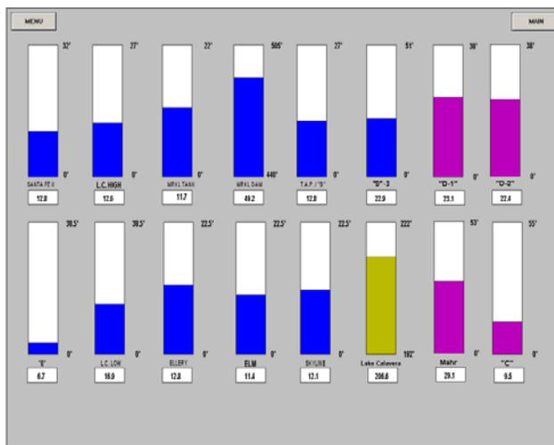
**HMI screens display the water levels of tanks, lakes, and reservoirs that supply the city.**
