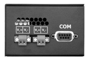
Unscrew & Remove the DC Voltage Input Plug(s) from the side header Install the DC Power Cables into the Plug(s) (observing polarity). Plug the Voltage Input Plug(s) back into the side header. Tightening torque for the terminal block power plug is **0.22 Nm/0.162 Pound Foot**. All LED's will flash ON Momentarily Verify the Power LED stays ON (GREEN).
