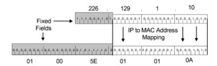
Mapping of class D 226.129.1.10 IP address to MAC layer multicast
