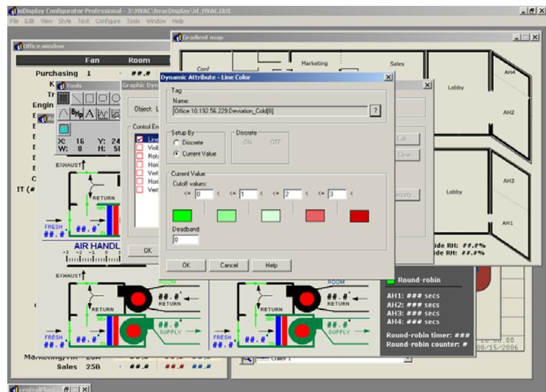
*HMI screens display HVAC equipment operation and color-coded representations of temperature setpoints compared to actual temperatures.*
