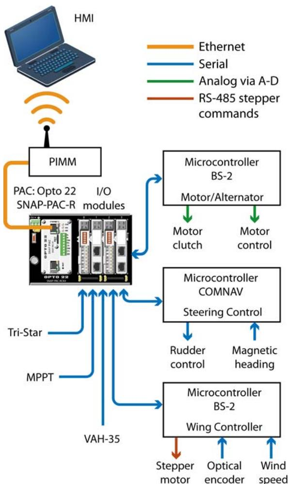
For example, a chart identified as "Captain" includes all the wind speed monitoring commands and executes the logic needed to determine when to turn the motor on and off, and at what speed it should run. The "Navigator" chart, meanwhile, uses data from the "Captain" as it performs the computations needed to determine the course to steer. The "Navigator" also gauges where the vehicle is with respect to where it's supposed to be.
