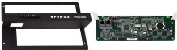
**G4D32EB2**—A complete Ethernet version of the G4D32RS *mistic* digital rack. Includes a G4EB2 brain, a G4 module mounting rack, a G4REG onboard regulator, and a metal cover.
