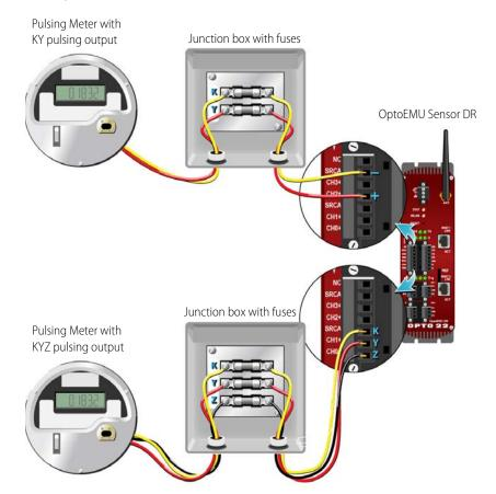
Use with either two-wire KY (Form A) or three-wire KYZ (Form C) pulsing devices.
