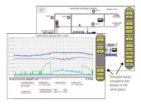
For consistency in SuperTrends, adjust the scales of trend pens so that they match, if possible. Scales that match make the trend more intuitive. For example, PID Setpoint and Input should have the same scale. Also adjust time scales so that they make sense and are readable in Runtime.
