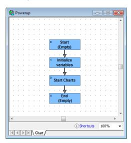
Add a block named End (empty) to the end of the Powerup chart (and other flow-through charts) just to make it clear that the chart stops. By the way, you don't need to put the Stop Chart command at the end of a chart; if there is no more logic, the chart will stop by itself.
