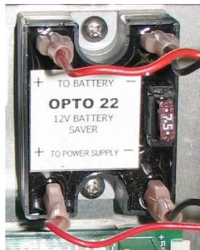
Unplug the existing cable that runs between the Battery Saver and the BAT connector on the modem board. Replace it with the supplied cable. You've finished the installation.
