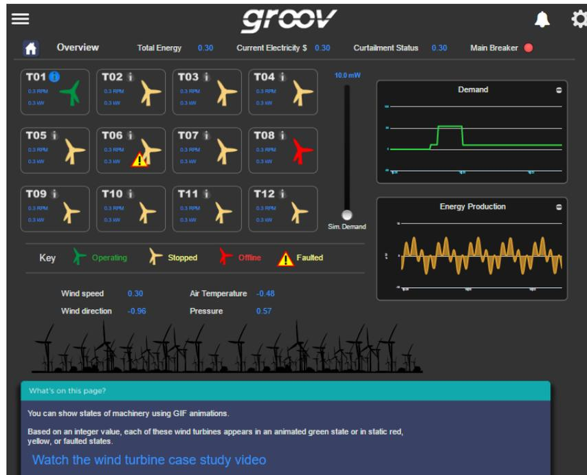
Here we see the states of several turbines. The color of the turbine indicates its state: green for operating, yellow for stopped, and red for offline. (The state of the turbines in your project may be different from those in this image.)
