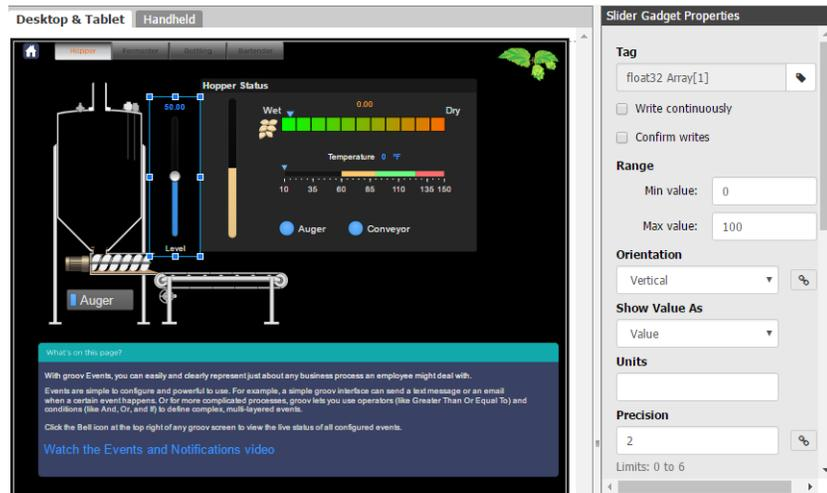
A control gadget is very much like an indicator gadget. The tag you’re controlling is at the top of the panel, with other properties below. You choose the appropriate range of values for whatever you’re controlling. You can orient this Slider gadget either vertically or horizontally on the page. You also control colors and labeling.
