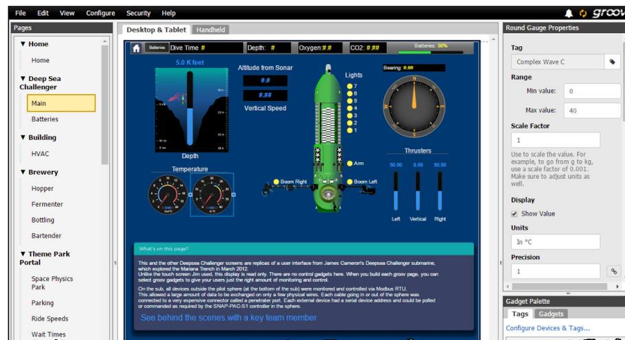
This is a Round Gauge gadget. When you click a gadget on the page in Build mode, you see its properties in the right-hand panel. As an Admin user in *groov* View, you can change these properties and add or delete gadgets. (For complete information on using Build mode, see the [groov View User's Guide](#).)
