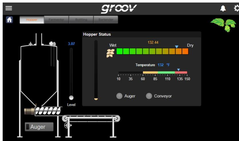
We're on the Hopper page, and here we can control the level of hops in the tank. We can also turn on the auger.
