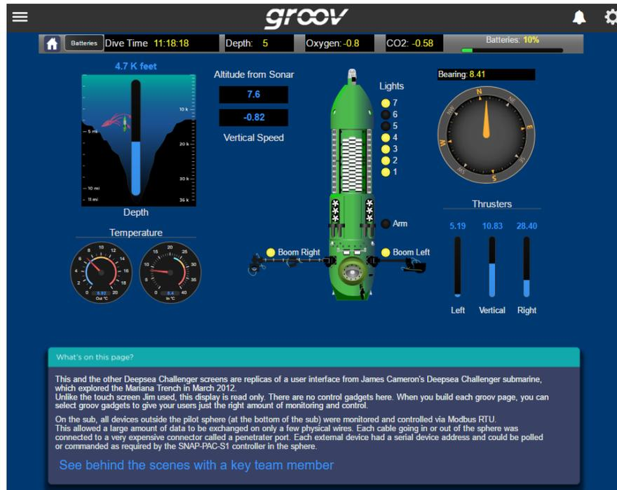
Notice how the compass at the right rotates based on the submersible's heading. You can build this kind of moving object using several images placed on top of each other. Let's see how it's done.
