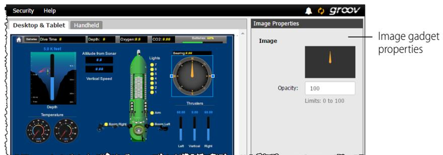
4. Go back to the compass in the workspace and drag it slightly to the right. Then click the image behind it. This is an Image Indicator gadget, and it's used to show a different image depending on the current value of the tag it represents.
