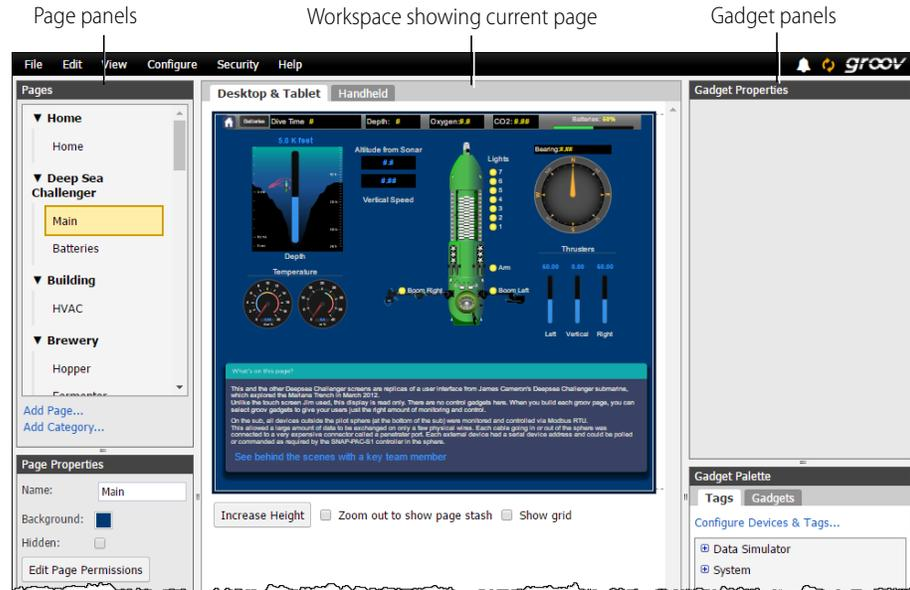
Each item on this page was built with one or more of the gadgets included in groov View. Each gadget is tied to a tag, which represents an I/O point to a physical sensor or device, a control variable, or a data item in software or equipment. Each gadget also has other properties—value details, colors, text, orientation, and a lot more—that you assign to it when you build the page.
