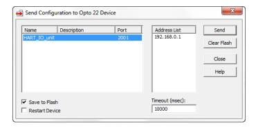
The list on the left shows all the I/O units in this configuration file. When you click a unit, the Address List shows the IP addresses for all I/O units to receive the same configuration.
