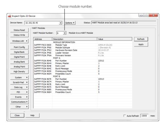
**8.** Set parameters for each port to match the HART device it will communicate with:
