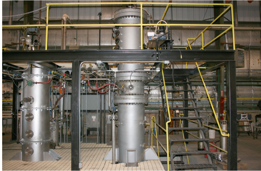
Figure 2: The pressurized fluidized bed gasifier processes solid fuels such as biowaste to investigate fuel reactivity, tar production, and quality of synthesis gas.
