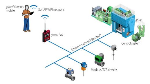
Again, the mobile devices on the SoftAP WiFi network have no direct connection with the automation equipment on the control network. Authorized employees on mobile devices who join the SoftAP network can see only the data and controls you've built into the *groov* interface.
