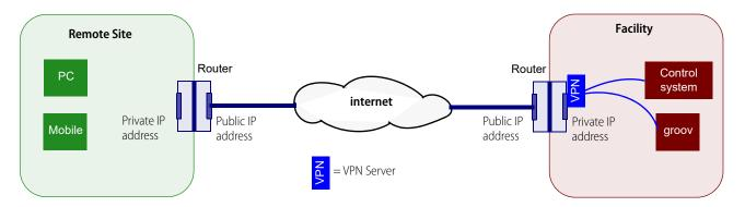
In the router, set up a port forward rule so the router will know to send data through the proper port to reach the VPN server. Port numbers depend on the VPN protocol you're using:
