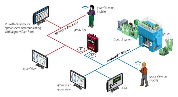
In this example, your *groov* Box is connected to your company computer network using ETH1 and to your control network using ETH0. (You could do the same thing with *groov* Server for Windows running on a PC that has two network interface cards.)
