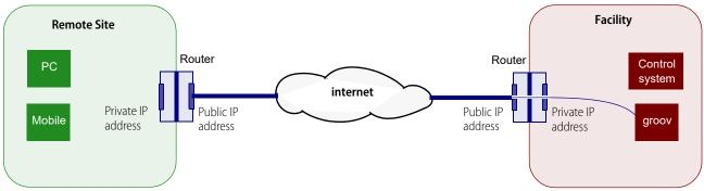
**Port forwarding** creates a hole in your firewall to allow certain packets through. PF works for *groov* because *groov* provides encryption and requires authentication from all users.
