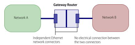
Software rules (routing tables, network address translation) determine whether and how communication moves between Network A and Network B.
