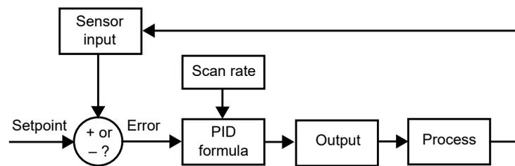
At the scan time, the sensor input is compared to the setpoint, and an error (the difference between them) is produced. This error is plugged into a mathematical formula with the P, I, and D components, and the result becomes the output that is then applied to the process. The sensor input is again compared to the setpoint, and the loop repeats.
