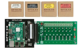
5. Remove an I/O module from its box and carefully install it in position 0 on the board. Secure it with its integral screw.
