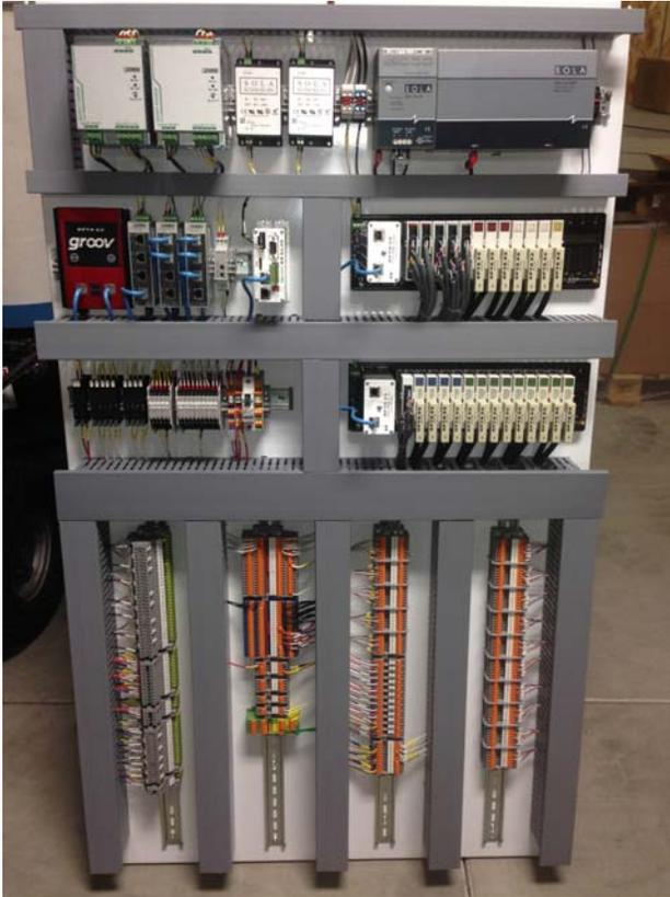
**Opto 22 PACs and I/O provide control and monitoring capabilities for ARi systems. Opto 22's *groov* provides remote monitoring and control, a common customer request.**
