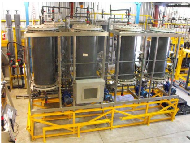
**Biomass SMB for recovery of basic sugars from cellulose waste**
