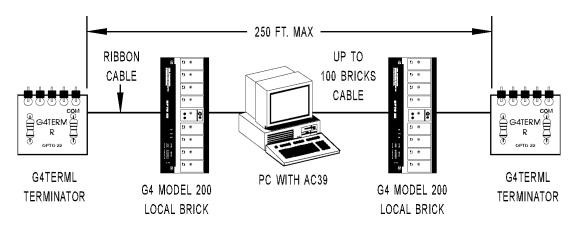
When AC39 is not at physical end of ribbon cable, you should install the G4TERML terminator at the two G4 Model 200 Local Bricks at the physical end of the cable.
