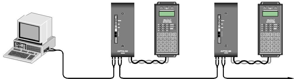
Figure 4-1: Fiber Optic Communications
