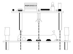
If you are attaching a B100 to a G4PB16J/K mounting rack, you must first attach a plastic, removable standoff to the brain board as shown in the figure above. Continue by installing the brain board to the mounting rack as described above and as shown in the figure to the left.
