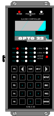
Remote Site PCAS Controller Figure 5
