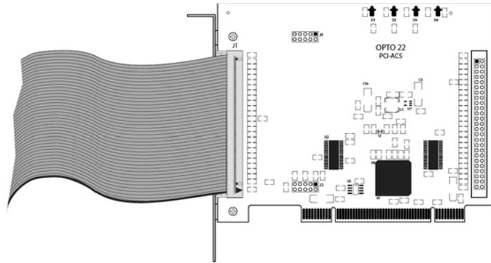
of the slot openings in the computer, and then attach the cable to the adapter card.
