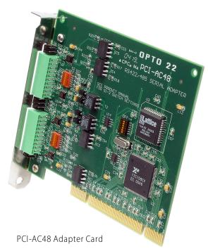
adapter card also provides tri-state control in hardware, 64-byte FIFO, and 16550 UART-compatible registers. The PCI-AC48 adapter card requires 5 VDC @ 600 mA and operates at temperatures of 0 °C to 70 °C. The card is configured using DIP switches. Six LEDs on the card indicate bus operation or user application status.
