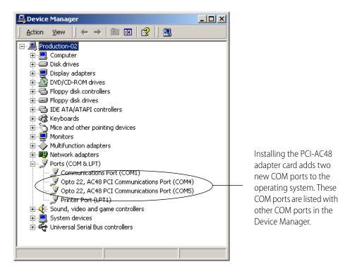
NOTE: The port numbers assigned to the adapter card's serial ports will vary depending on the number of COM ports that the computer system has.
