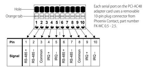
IRQ + and IRQ - are optional inputs that can be used with mistic I/O systems to trigger an interrupt. For more information, see "Using External Interrupts for mistic Remote I/O" on page 19.
