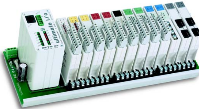
Opto 22's SNAP Ultimate I/O System: Brain, Modules, and Rack
