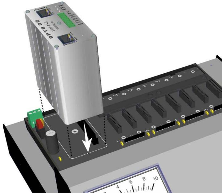
3. Seat the controller onto the connector.
