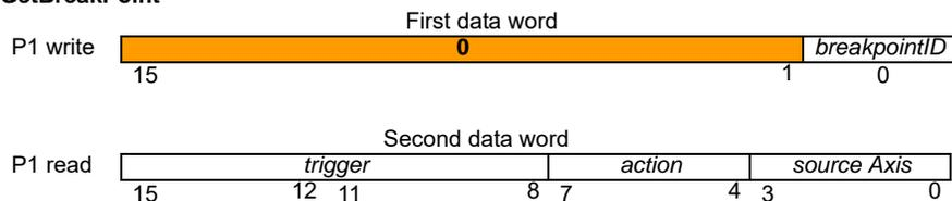
**Description** SetBreakPoint establishes a breakpoint for the specified axis to be triggered by a condition or event on sourceAxis, which may be the same as or different from axis. Up to two concurrent breakpoints can be set for each axis, each of which may have its own breakpoint type and comparison value. The breakpointID field specifies which breakpoint the SetBreakPoint and GetBreakPoint commands will address.
