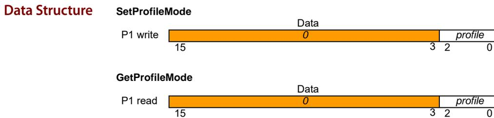
**Description** SetProfileMode sets the profile mode for the specified axis.
