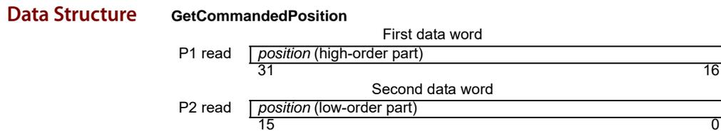
**Description** GetCommandedPosition returns the commanded position for the specified axis. Commanded position is the instantaneous position value output by the trajectory generator.
