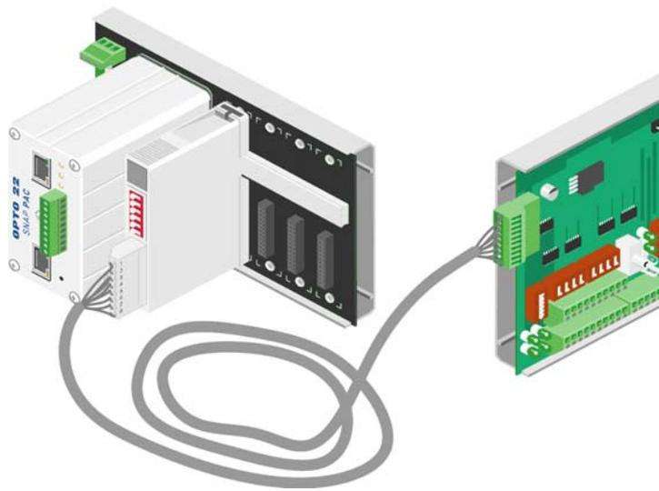
6. Connect your stepper motors to the SNAP-SCM-BB4. Minimum connections are Pulse, Direction, and GND. Make sure you have a power supply for the stepper motor. To locate the connector pins on the board, see [“Breakout Board Connector Pins”](#) on page 8.
