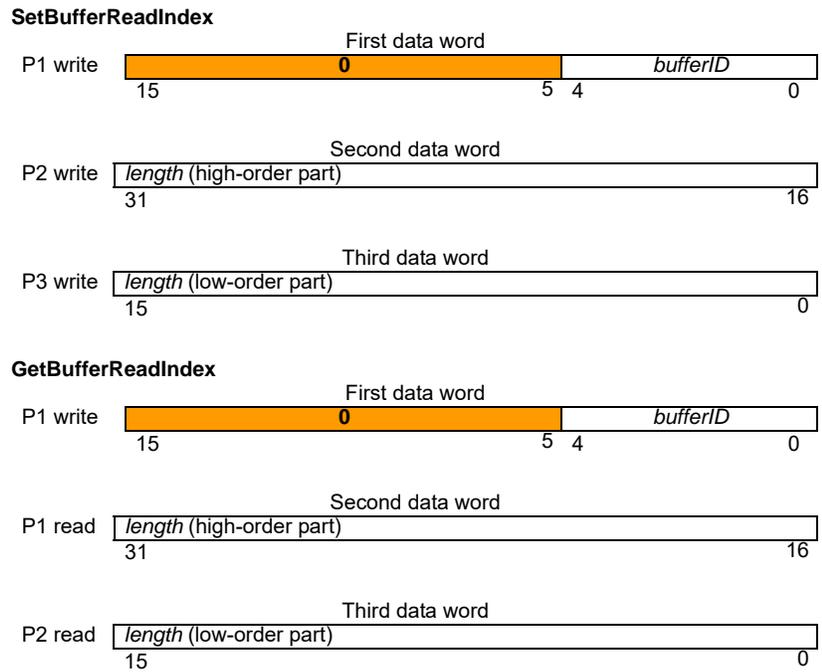
**Description** SetBufferReadIndex sets the address of the read index for the specified bufferID. GetBufferReadIndex returns the current read index for the specified bufferID.
