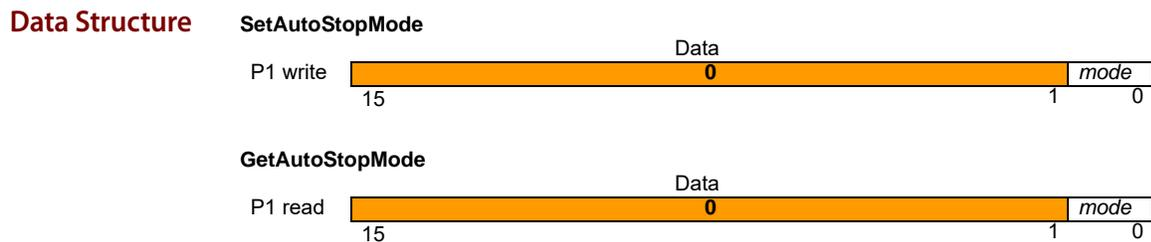
**Description** SetAutoStopMode determines the behavior of the specified axis when a motion error occurs. When auto stop is enabled (SetAutoStopMode Enable), the axis goes into open-loop mode when a motion error occurs. When Auto-Stop is disabled (SetAutoStopMode Disable), the axis is not affected by a motion error.
