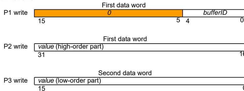
**Description** WriteBuffer writes the 32-bit value into the location pointed to by the write buffer index in the specified buffer. After the contents have been written, the write index is incremented by 1. If the result is equal to the buffer length (set by SetBufferLength), the index is reset to 0.
