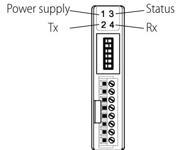
*Power Supply Fault* indicates a fault on the internal power supply of the module (too much draw). This will happen if more than one breakout board is connected without additional power supplies, or there is a short in the system.
