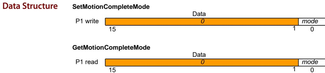
**Description** SetMotionCompleteMode establishes the source for the comparison which determines the motion complete status for the specified axis. When set to commanded mode the motion is considered complete when the profile velocity reaches zero and no further motion will occur without an additional host command. This mode is unaffected by the actual encoder location.
