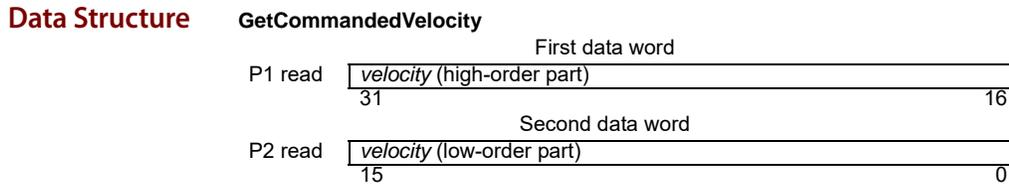
**Description** GetCommandedVelocity returns the commanded velocity value for the specified axis. Commanded velocity is the instantaneous velocity value output by the trajectory generator.
