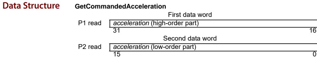
**Description** GetCommandedAcceleration returns the commanded acceleration value for the specified axis. Commanded acceleration is the instantaneous acceleration value output by the trajectory generator.
