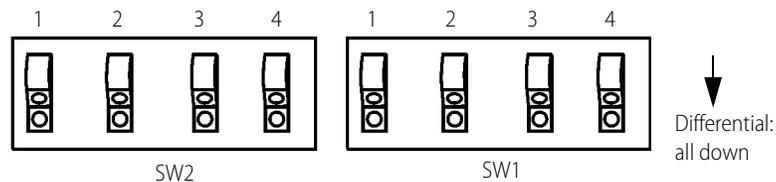
If your encoder outputs non-differential signals, make sure they are in the Non-Differential Signals position: all *up*.
