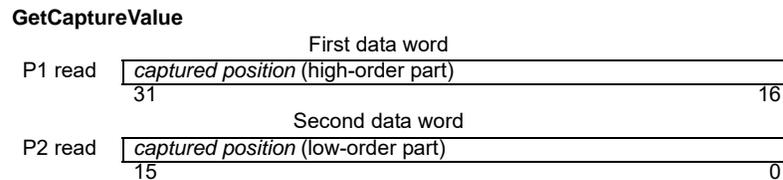
**Description** GetCaptureValue returns the contents of the position capture register for the specified axis. This command also resets bit 9 of the activity status register; thus allowing another capture to occur. If actual position units is set to steps, the returned position will be in units of steps.
