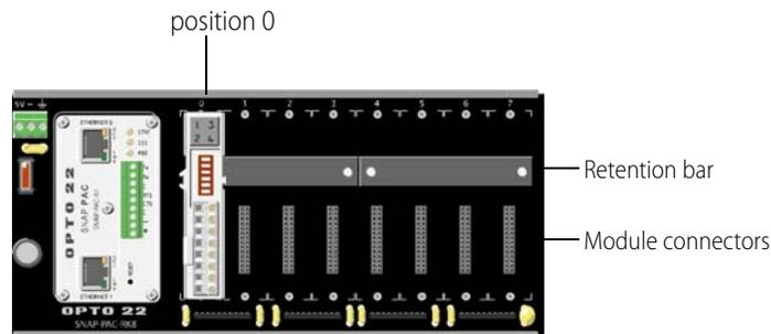
4. With the module correctly aligned over the connector, push on the module to snap it into place.
