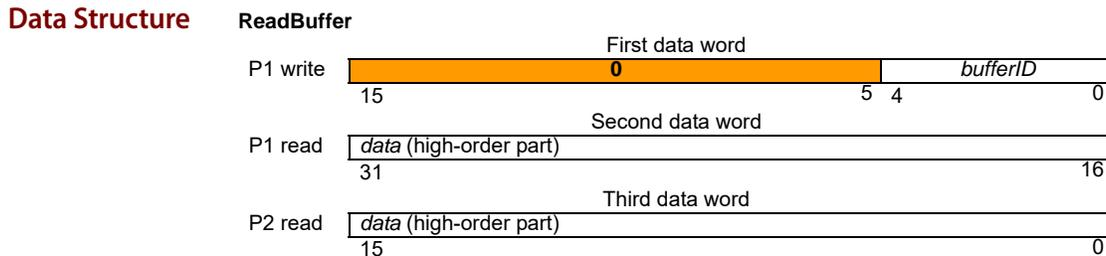
**Description** ReadBuffer returns the 32-bit contents of the location pointed to by the read buffer index in the specified buffer. After the contents have been read, the read index is incremented by 1; if the result is equal to the buffer length (set by SetBufferLength), the index is reset to 0. The read index is automatically changed at the completion of a trace when in rolling trace mode.
