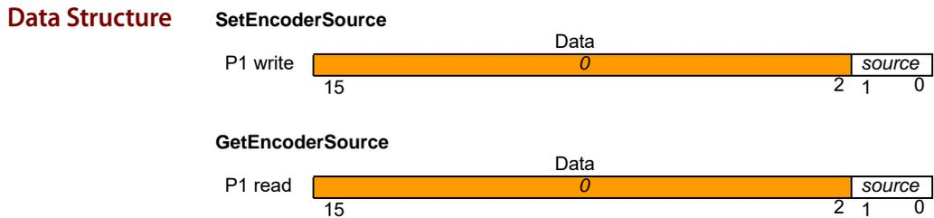
**Description** SetEncoderSource sets the type of feedback (Incremental, None, or Loopback) for the specified axis. When incremental is selected the motion processor expects A and B quadrature signals to be input at the quad A/B axis inputs. When Loopback is selected, the step output is internally fed back into the quad counters. This allows for position capture of the step position when a physical encoder is not present.
