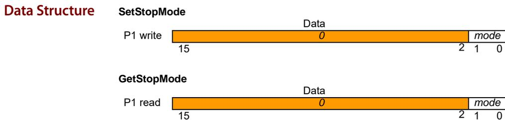
**Description** SetStopMode stops the specified axis. The available stop modes are AbruptStop, which instantly (without any deceleration phase) stops the axis, SmoothStop which uses the programmed deceleration value and profile shape for the current profile mode to stop the axis, or Disabled, which is generally used to turn off a previously issued set stop command.
