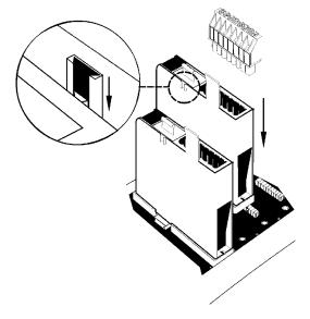
**5.** As shown in the photo at right, use the hold-down screws to secure both sides of each module.
