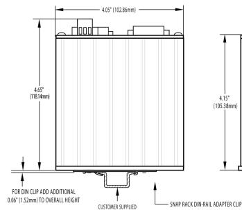
35mm DIN RAIL NOTE: BESURE TO CONSIDER DIN RAIL DIMENSIONS.
