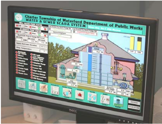
HMI screens were developed to give Waterford personnel visual representations of equipment and processes and point-and-click control capabilities.
