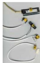
**Thermistors** work by offering resistance that varies with the temperature. In this and other ways, thermistors work very much like RTDs, but they differ in that thermistors use 2-wire interconnections that are more sensitive to temperature. This makes thermistor readings somewhat less than precise. Additionally, the material used in
