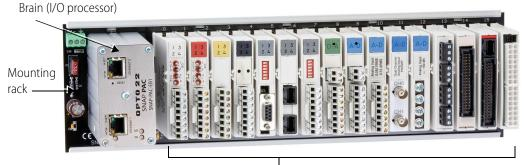
I/O modules (analog, digital, serial)
