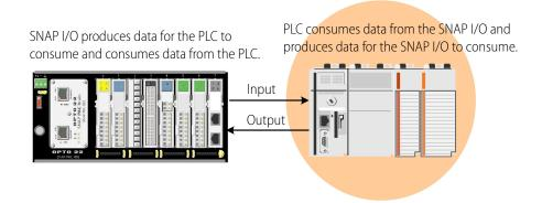
So for each implicit messaging connection, there are two producer-consumer relationships, one for each direction of data flow. To accomplish this double data flow, the data structures are defined by creating assembly instances.
