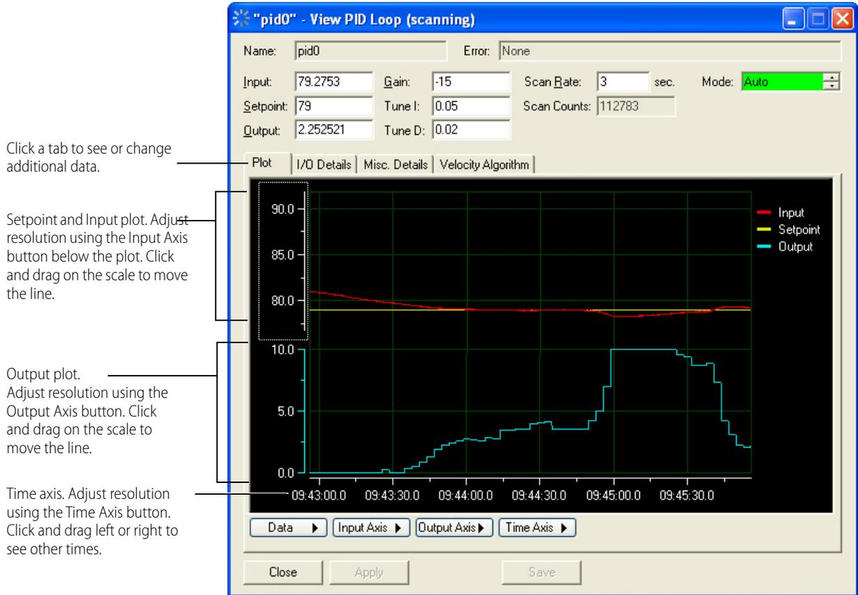
3. View or change PID parameters as necessary. Click the other tabs to see additional data. To tune the PID, see [page 86](#).
