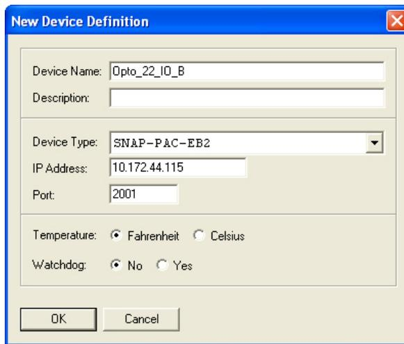
**Device Name.** Enter a name for the remote I/O. The name must start with a letter and may contain letters, numbers, and underscores. (Spaces are converted to underscores.)
