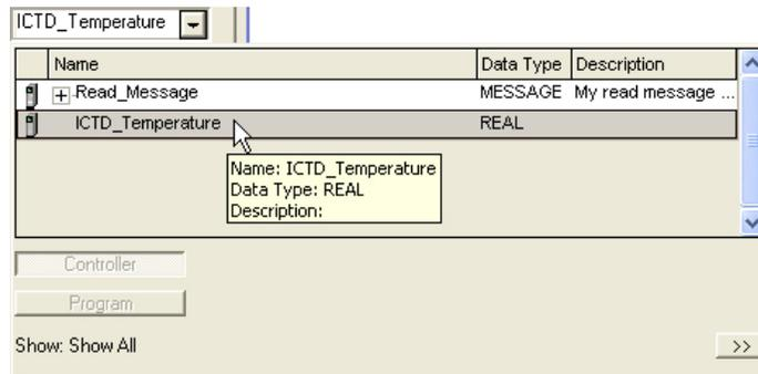
The configuration tab shows a list of tags with the following columns: Name, Data Type, and Description.
