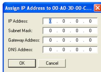
4. Enter the IP Address and the Subnet Mask for the device. If it will be talking to a device on another subnet, enter the Gateway (router) address. If it will talk only on the local subnet, leave the gateway address all zeros (0.0.0.0). Leave the DNS address at 0.0.0.0 field blank.
