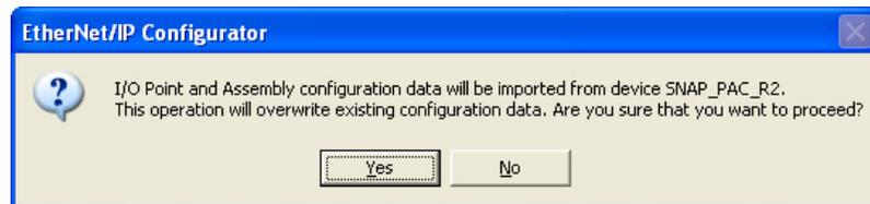
3. Click Yes to upload the configuration data. This action overwrites the device's existing configuration data for any module position that is the same as the new configuration data.
