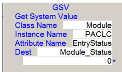
The GSV instruction may add a burden to the ladder's scan time. As a result, the detection of I/O failures should be implemented efficiently. Consider using a timer as a time period check to evaluate the status of the PLC's I/O indicator. If this indicator should indicate a failure, then a routine should be called to test the status of the I/O units. Calling a routine after knowing there is a failure will reduce the number of GSV and conditional tests the ladder will have to perform.
