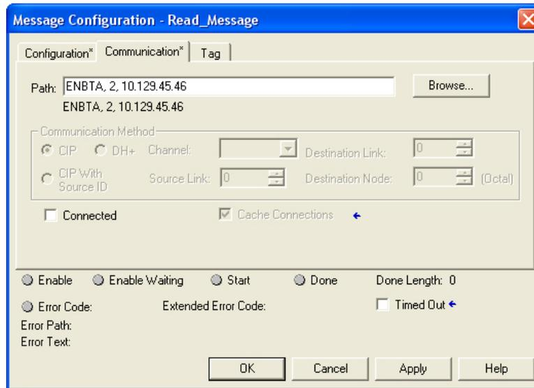
For a CompactLogix controller (1769-32E) with an embedded EtherNet/IP Communication module, the path changes slightly. RSLogix automatically names the embedded EtherNet/IP module "LocalENB." All other values of the path are the same.
