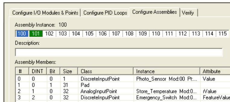
EtherNet/IP Configurator indicates the size of the assembly instance at the bottom of the screen as shown here.
