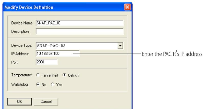
This is important because the imported configuration will likely have the local loopback address for the I/O unit (127.0.0.1) instead of the IP address for the PAC R. In order to communicate with the PAC R, EtherNet/IP Configurator needs the device's IP address.
