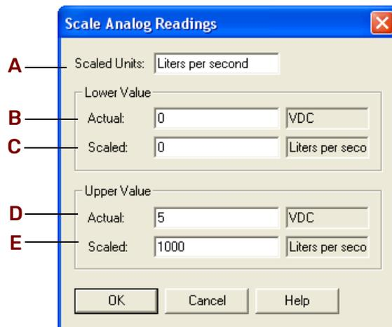
This example shows units scaled to liters per second. At an actual input of 0 VDC, the point will show 0 liters per second. At an actual input of 5 VDC, the point will show 1000 liters per second.
