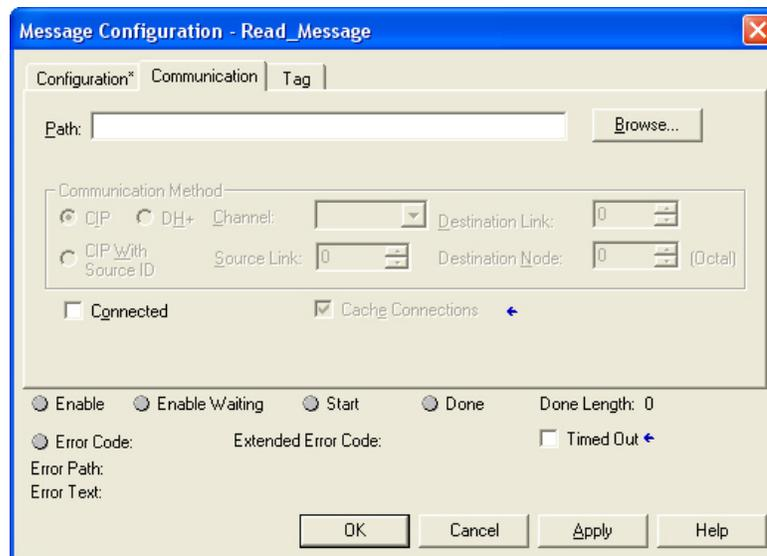
12. For a ControlLogix controller (1756-L61 with a 1756-ENBT/A) implementation, enter the communication path, **ENBTA, 2, 000.000.000.000**, where:
