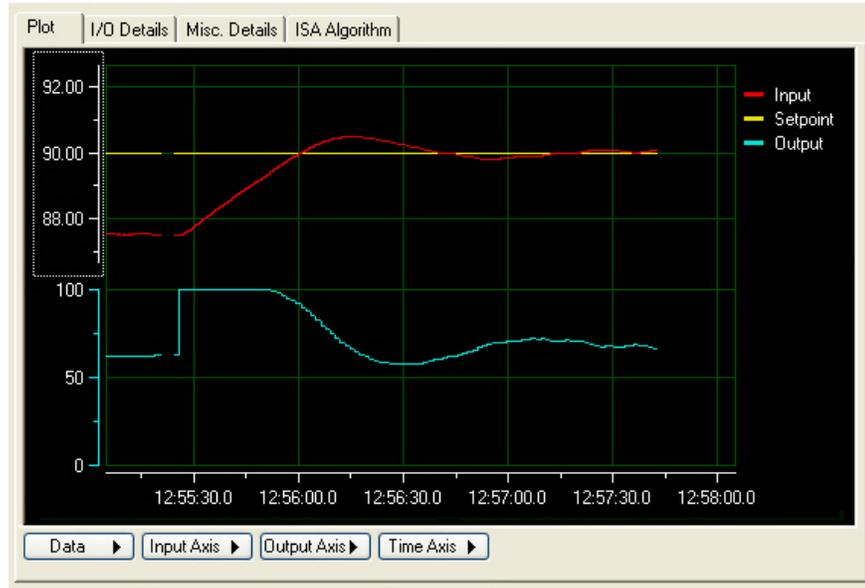
10. If derivative correction is needed, experiment with the derivative constant: in the Tune D field, type 1 and click Apply. (Your PID loop may require a larger number.)
