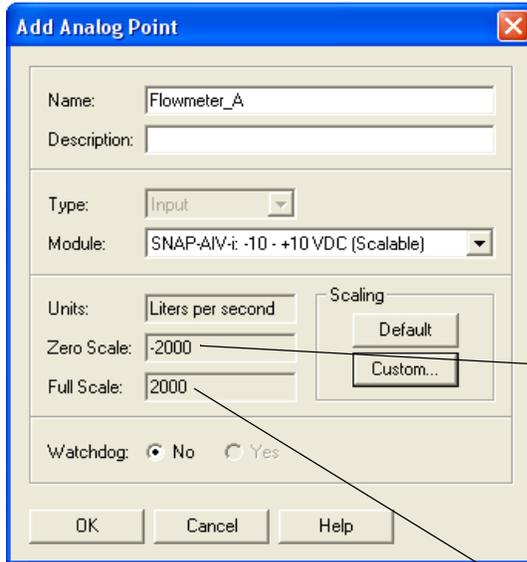
Notice the new units of liters per second and the new minimum-scale (“Zero Scale”) and maximum-scale (“Full Scale”) values of -2000 and +2000. The example connects a sensor with a range of 0–1000 liters per second, but an output of only 0–5 volts, to a SNAP-AIV module with an output of -10 to +10 volts. The figures shown in this dialog box reflect the total possible range of the module, not the sensor.
