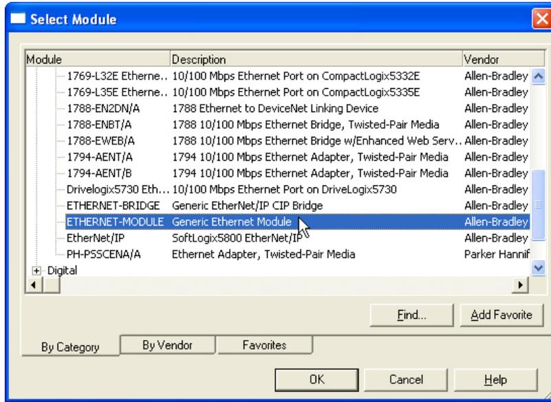
8. Scroll down to Generic Ethernet Module and then double-click it to open the New Module dialog box.
