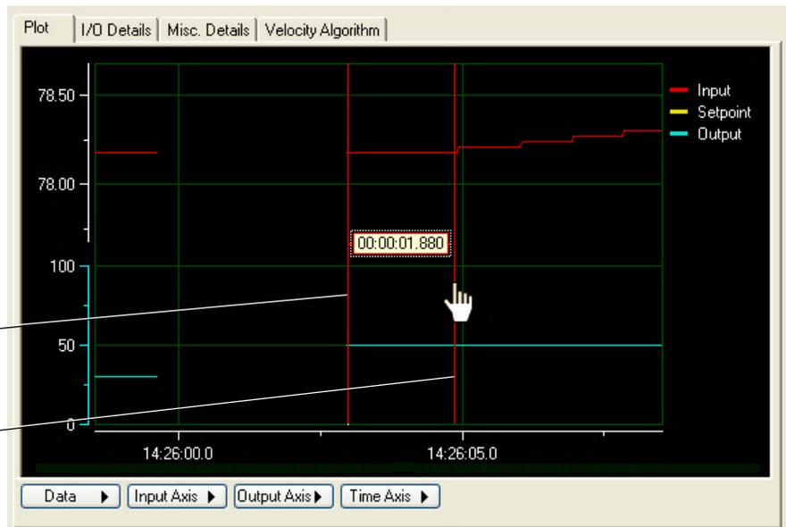
If you are unable to get the precision you want, you can view the plot at a lower time span, such as 10 seconds. You will need to reposition your plot and the measurement bars of the Delta X cursor.
