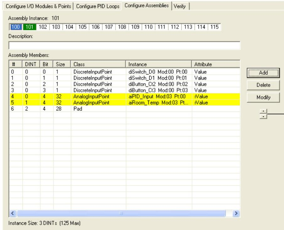
To move the pad, select it and click the appropriate arrow to move the pad into its proper place.
