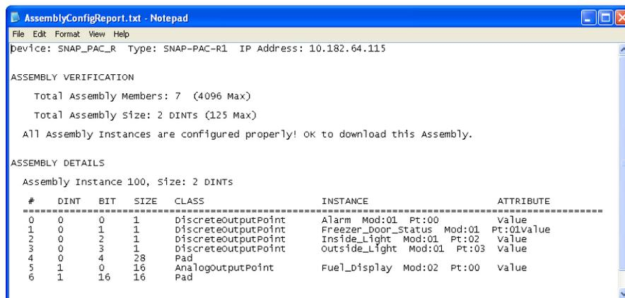
The *I/O Modules and Points Configuration Report* lists the modules and points configured for the selected device.
