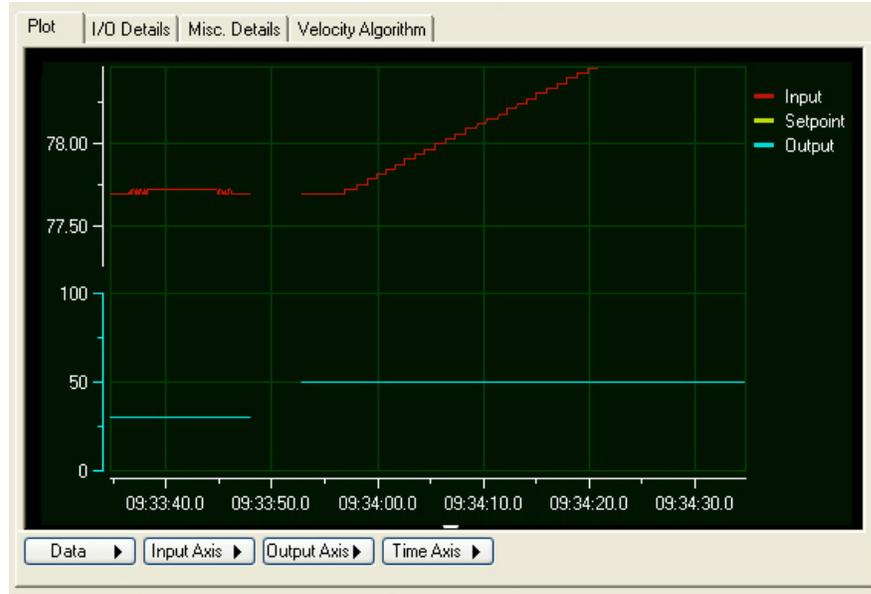
15. From the Data menu, select Cursor. The data cursor, a line with a value bar attached to it, appears on the plot.
