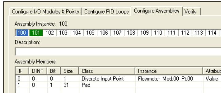
The following example assembly from EtherNet/IP Configurator has three 32-bit words, so you would enter a size of 3 in RSLogix 5000.
