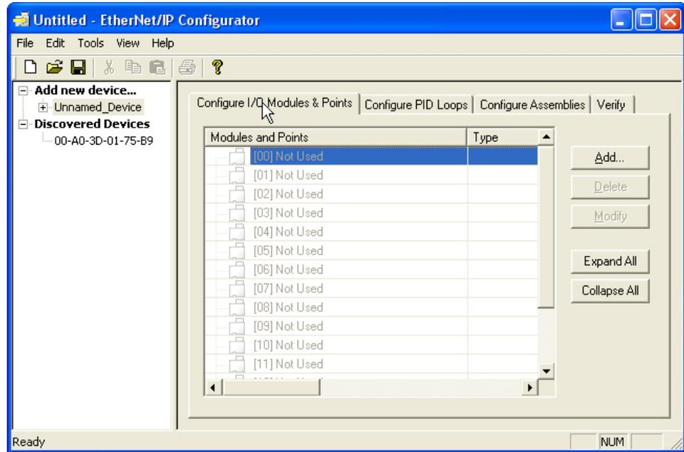
2. Double-click the number that represents the digital module's position on the rack. For help, see ["Referencing I/O Points on SNAP PAC Racks"](#) on page 93.
