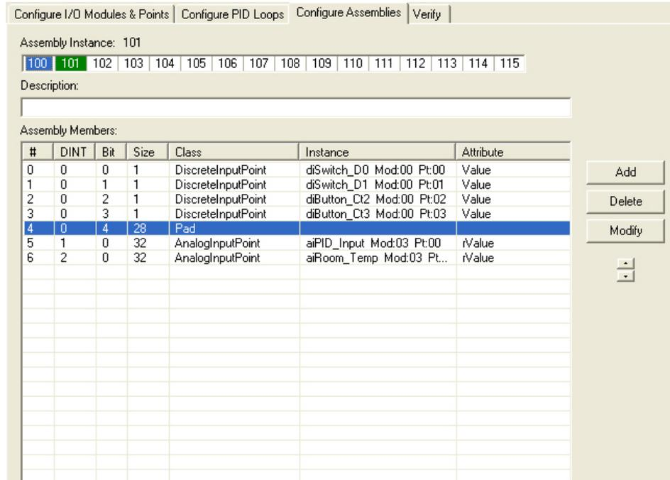
The input assembly instance is now once again formatted properly with 32-bit words.
