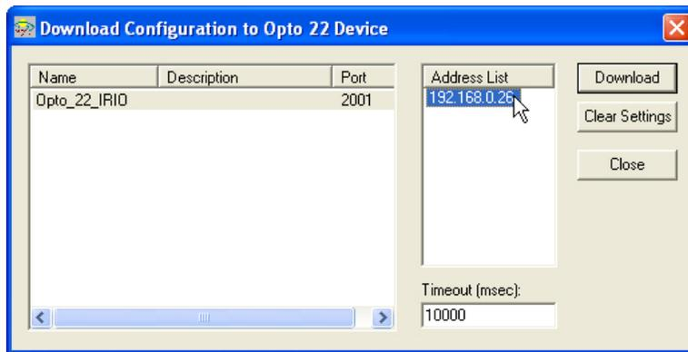
This completes the setup of the Opto 22 remote I/O for implicit messaging. In the next section, you will configure communications with the Allen-Bradley controller.
