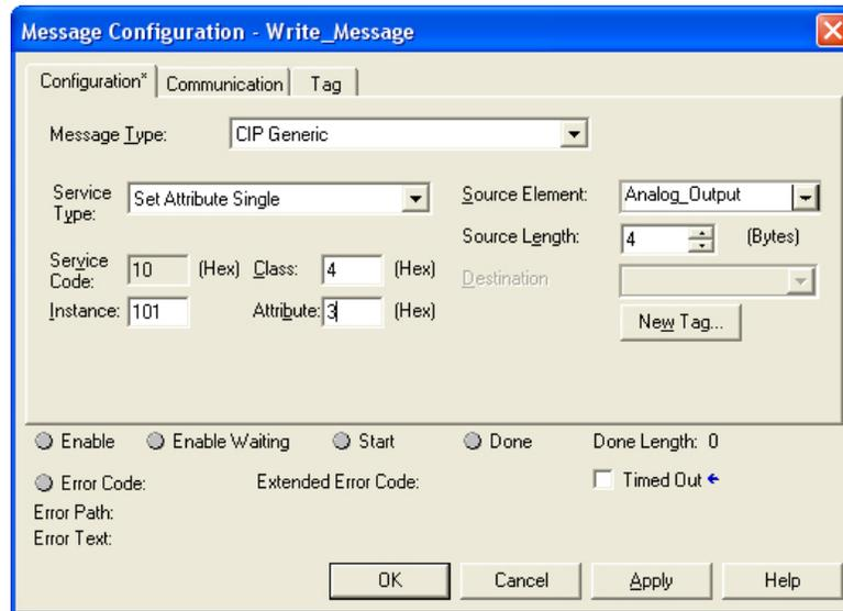
Note that this message is an Opto 22 Object Model Class 0x04, attribute 0xe, and references the assembly instance 101, where the output is configured.
