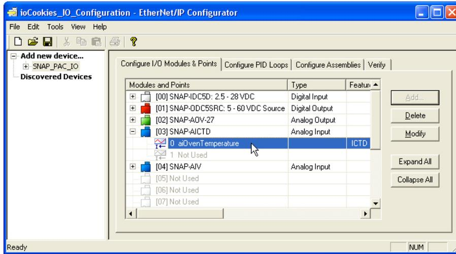
3. Click the Configure Assemblies tab, select assembly instance 100, and click the Add button to open the Add Assembly Member dialog box.
