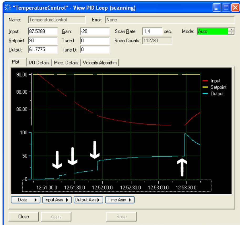
In this example, a gain setting of -30 revealed an offset error:
