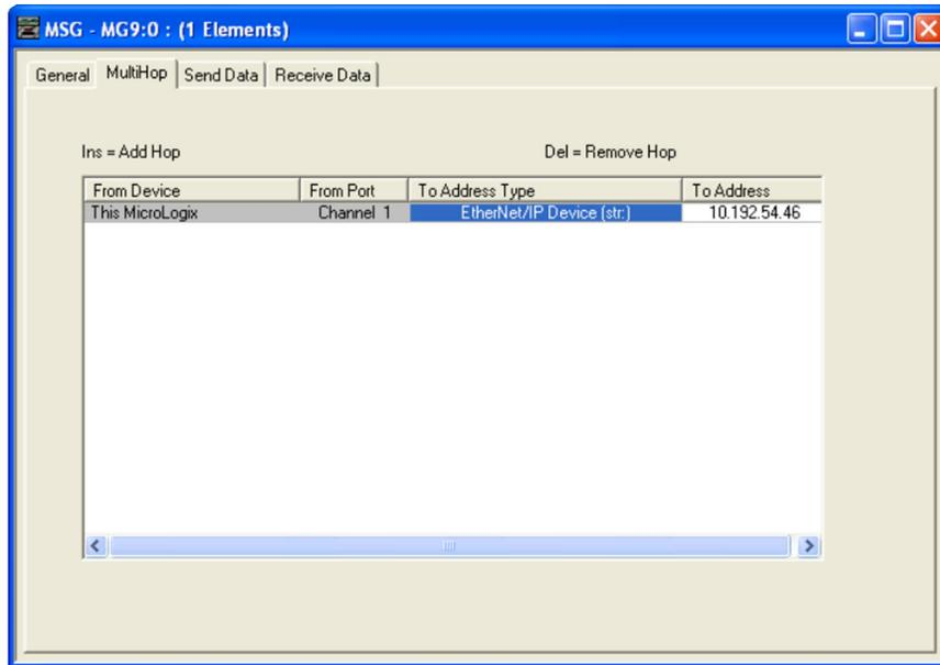
The MSG has a limit of 124 16-bit words. However, when working with the EtherNet/IP Configurator, there is a lower limit for each assembly. For the MicroLogix family, an assembly instance may not exceed 62 DINTs (32-bit integers).
