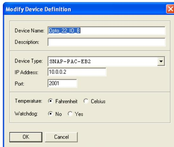
*NOTE: Changing the IP address in this dialog box does not change the IP address on the device. If you want to change the IP address on the device, see ["Changing a Device's IP Address"](#) (below).*
