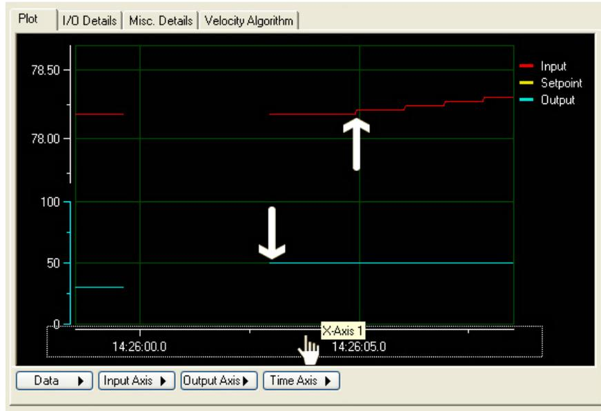
13. Increase the resolution of the Time Axis by clicking the Time Axis button and choosing a lower percentage, such as View 1 Minute Span.
