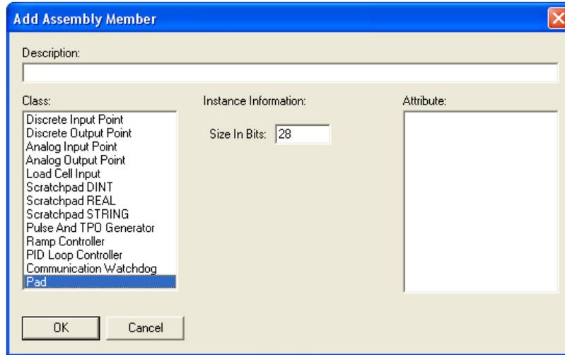
The pad appears as the last member of element 0 to complete the 32-bit word, also called a DINT. You can add up to 125 input DINTs.
