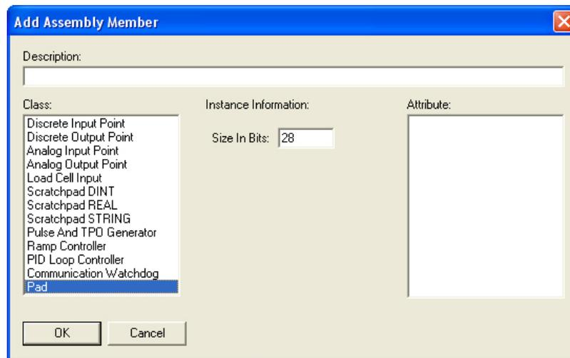
The pad appears as the last member of element 0 to complete the 32-bit word (or DINT). You can add up to 124 output DINTs.
