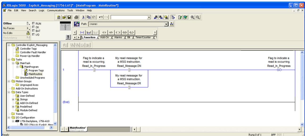
Rung 1 in this example is incomplete. When the XIC for Read\_Message.DN closes, the explicit data read is available. If the Explicit Message fails, the XIC for Read\_Message.ER will close. In either case, the typical ladder implementation will add additional logic to handle both successful and unsuccessful communications.
