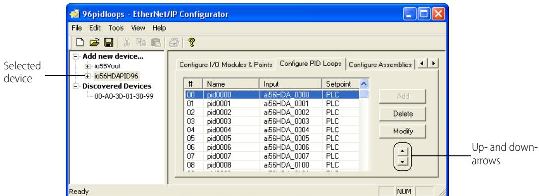
PID loops are scanned by the I/O unit in the order that they appear in this list.
