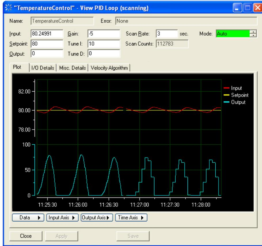
8. Experiment with gain settings by typing a new value in the Gain field and clicking Apply. The easiest way to tune most PIDs is to experiment with the gain constant first. Try various gains to see how well the system stays at setpoint and responds to setpoint changes. The white arrows in the example below show where gain constants of -2, -5, -10, and -20 were applied:
