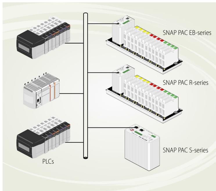
**EtherNet/IP automation environment with PLCs and Opto 22 devices**
