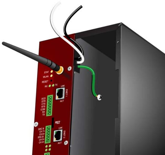
4. Connect Load to the black wire and Neutral to the white wire. Connect ground to the grounded chassis (see label inside box).
