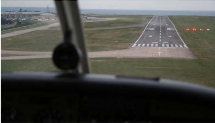
**PAPI systems have an effective visual range of at least 3 miles during the day and up to 20 miles at night. Light combinations indicate when slightly high (3 white ●●●), significantly high (4 white ●●●●), slightly low (3 red ●●●) and significantly low (4 red ●●●●).**
