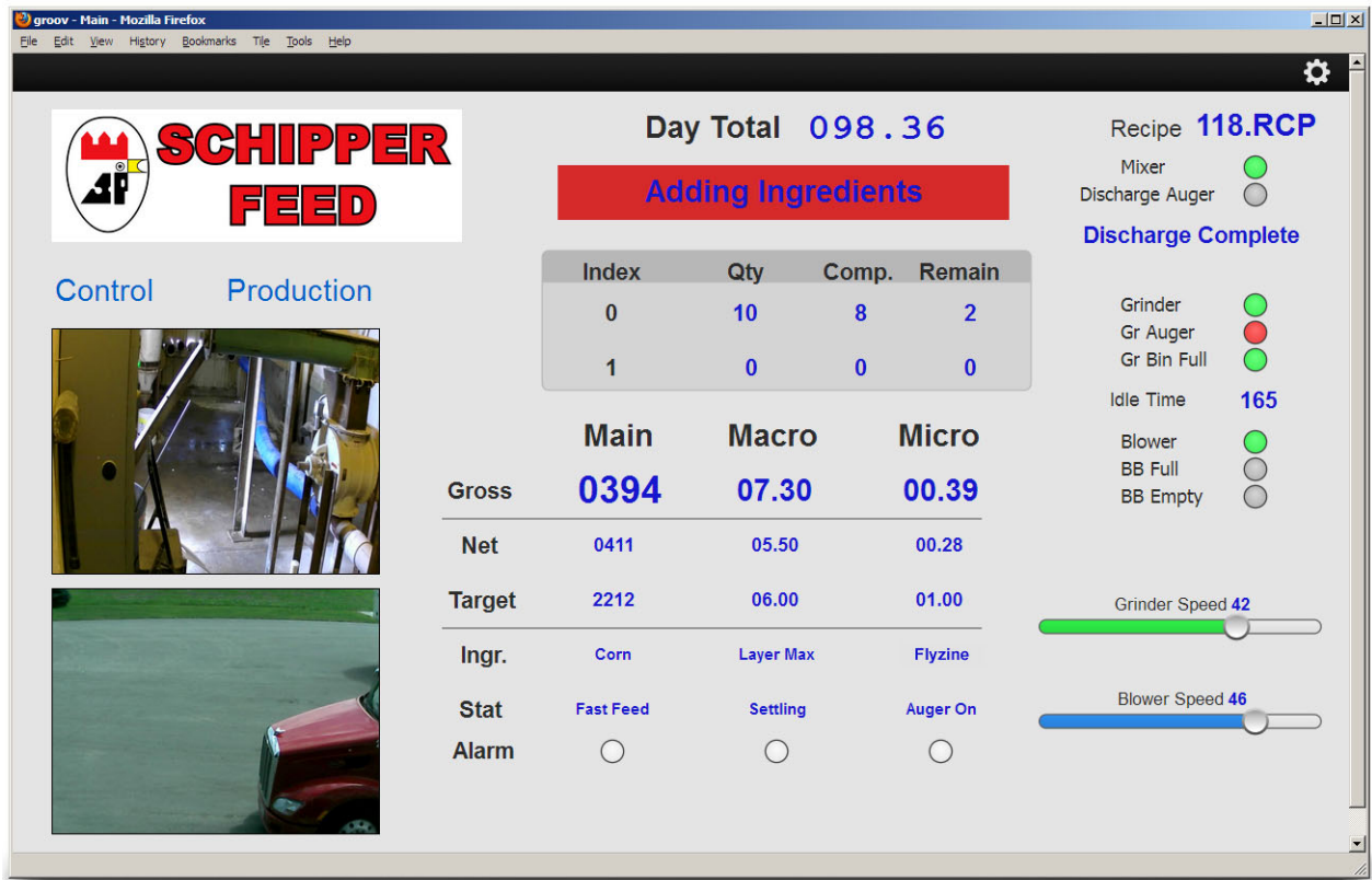
A web-browser-based display includes live video in an overview of machinery status.
