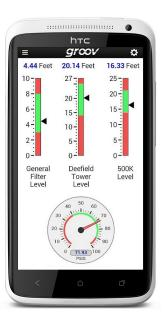
Tank levels and pressures are readily available on a smartphone.
