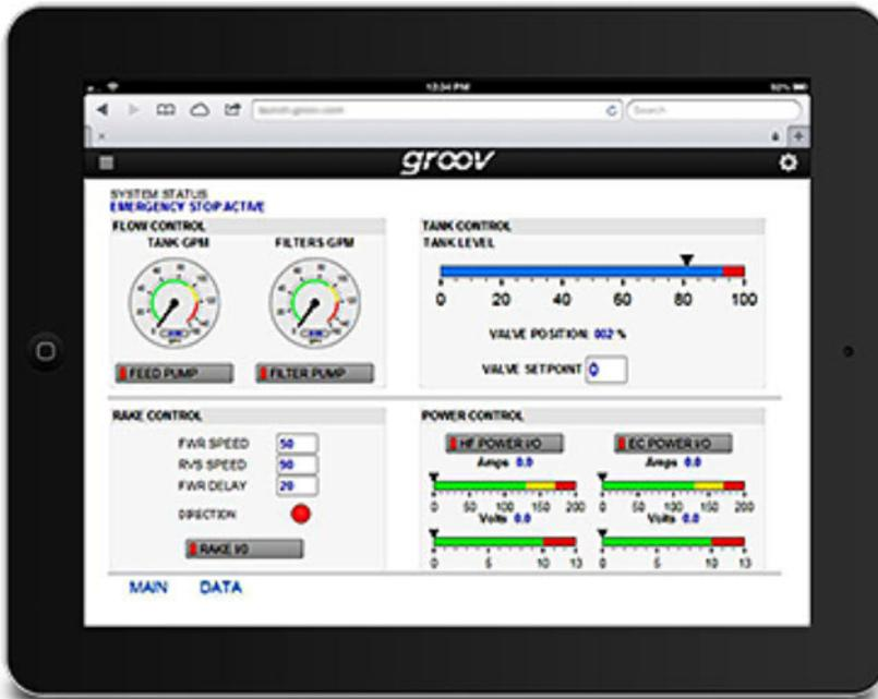
Key parameters for a mobile water treatment system are monitored and controlled using a tablet.
