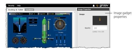
**4.** Go back to the compass in the workspace and drag it slightly to the right. Then click the image behind it. This is an Image Indicator gadget, and it's used to show a different image depending on the current value of the tag it represents.
