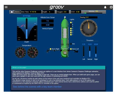
Notice how the compass at the right rotates based on the submersible's heading. You can build this kind of moving object using several images placed on top of each other. Let's see how it's done.
