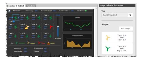
The image of the yellow turbine is static, but the image of the green turbine is moving. The yellow turbine is a PNG file, but the green turbine is an animated GIF. If you hover your mouse over the image in the Properties panel, you can see the name of the file. All image files are stored in the Image Library. For more on the Image Library and on using all gadgets, see the *groov* View User's Guide.
