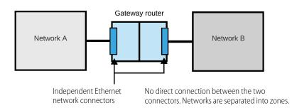
Software rules (routing tables, network address translation) determine whether and how communication moves between Network A and Network B.
