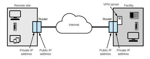
In the router, set up a port forward rule so the router will know to send data through the proper port to reach the VPN server. Port numbers depend on the VPN protocol you're using:
