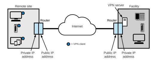
Most current PCs and mobile devices have VPN client software built in. The VPN client must use the same VPN protocol as the VPN server. Some clients give you a choice.
