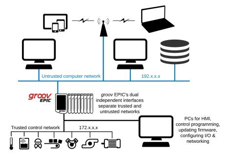
NOTE: It doesn't matter which wired interface you use for each network, except that when you first plug a groov EPIC into the network, you must use its lower-numbered interface for initialization.
