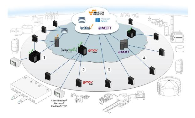
In area 1, a shared infrastructure with edge data processing links several remote locations to central software. In area 2, legacy PLCs are integrated with current I/O systems and all data sent to the cloud using a *groov* EPIC processor as an IoT gateway.
