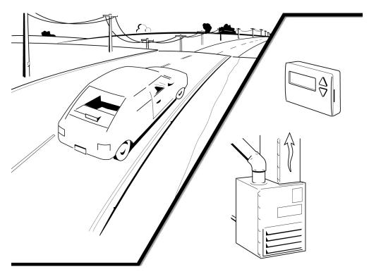
• **Room thermostat.** In the case of the room thermostat, the temperature is measured and compared to the desired setpoint. Either heating or cooling will be activated, depending on the sign of the error.
